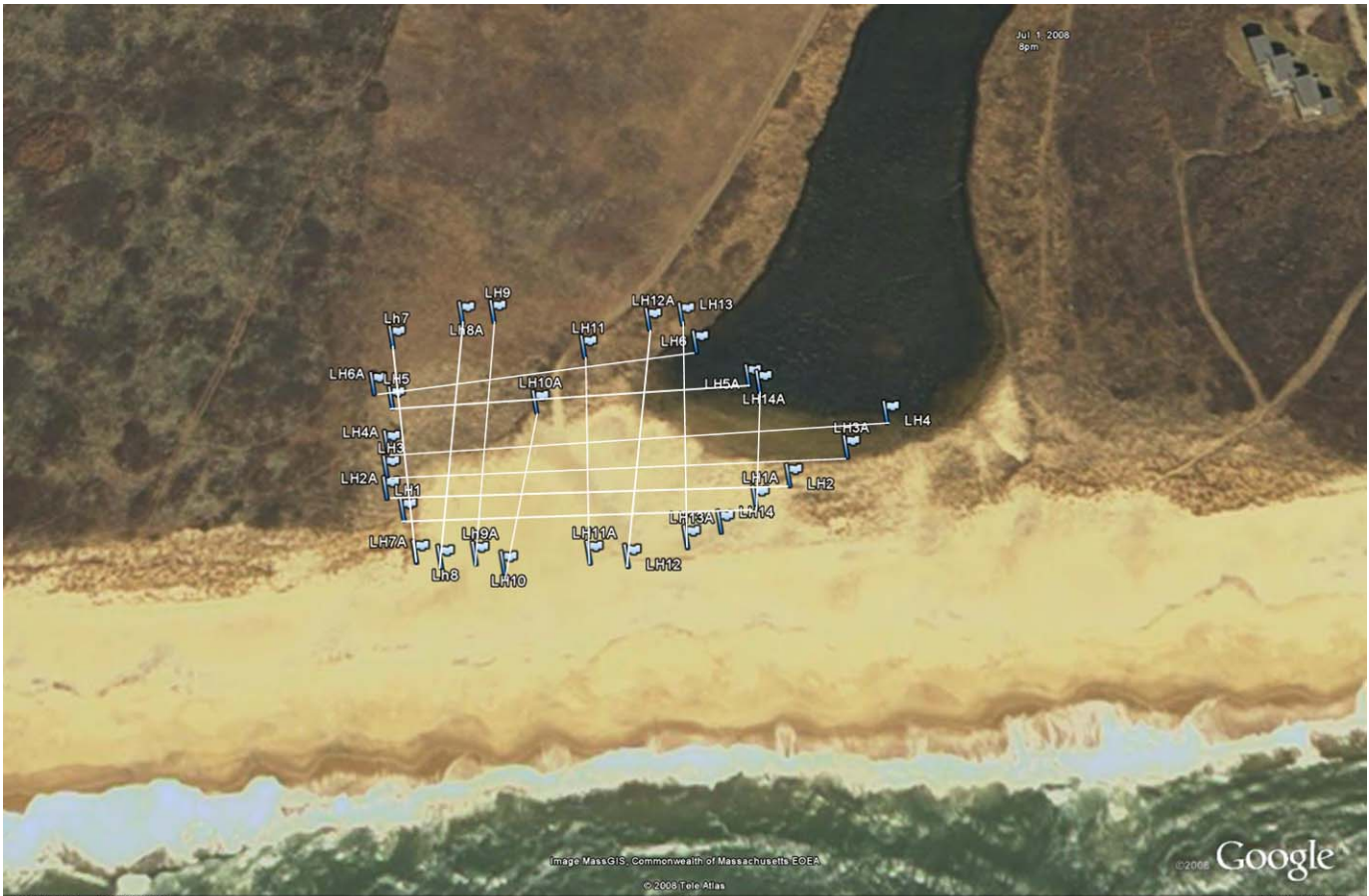
Figure 6. (a) Location map of the two GPR study sites, southeastern Massachusetts. (b) Map showing the grid of transects taken at Little Homer Pond, Martha's Vineyard.
