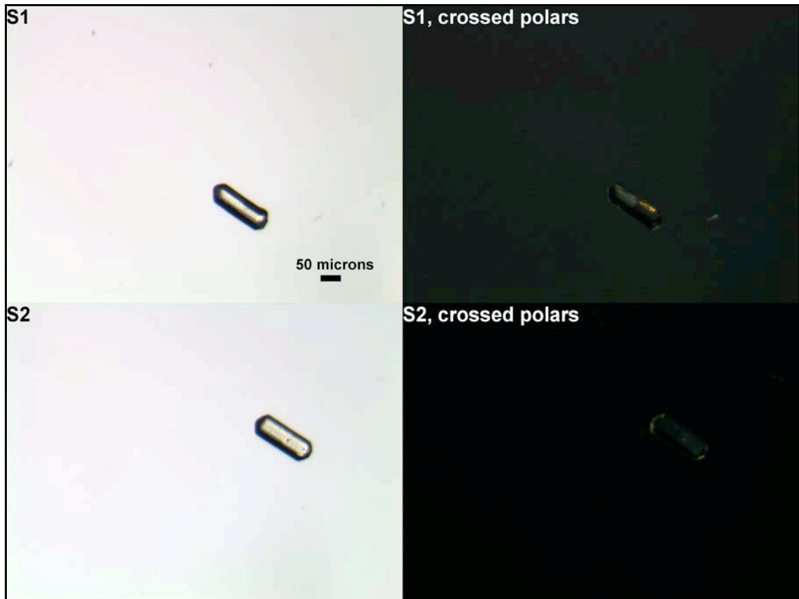
Appendix Figure A1: An apatite crystal from sample with few inclusions and nicely formed ends. Grain is about 70 microns across.
