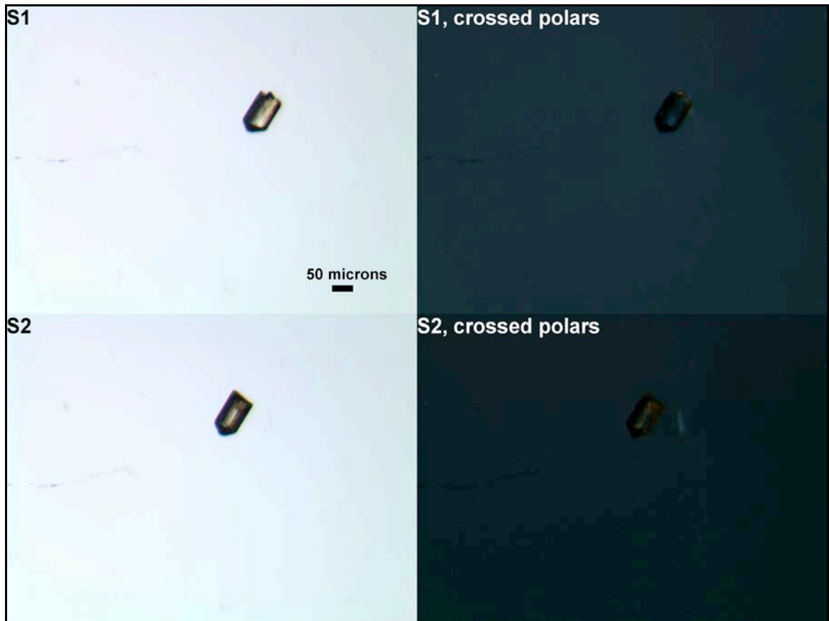
Appendix Figure A2: Many crystals had fractured ends or inclusions, but were chosen because they were the best the sample contained.
