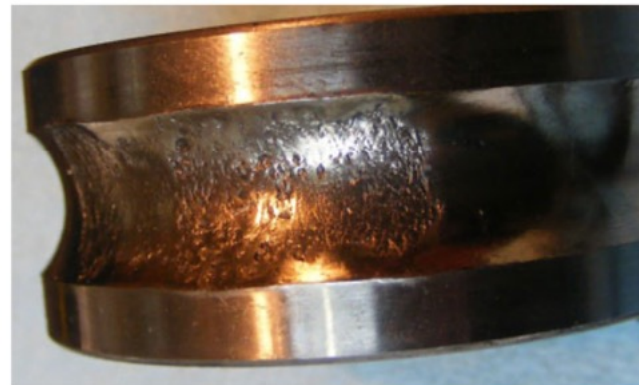
↑ (CLOCKWISE FROM TOP LEFT) Circuit diagram of the rotor's capacitive couplings between the coils, shaft, and frame. Illustration of the capacitive couplings responsible for EDM in a bearing system. Pitting on the surface of a ball bearing caused by EDM. Fluting on the outer raceway of a ball bearing caused by EDM.
