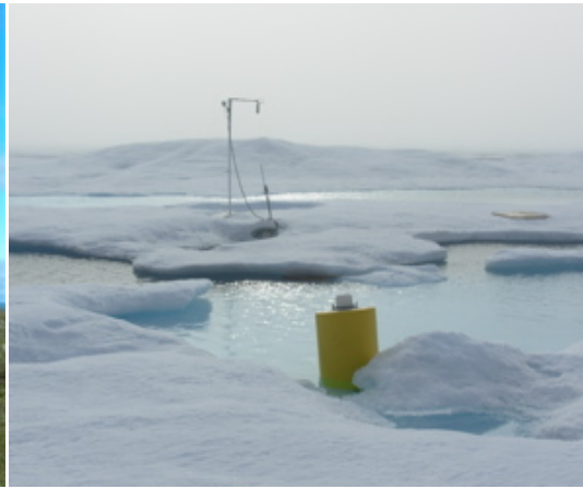
Figure 1b. IMB thermistor string in the distance, where temperature is measured 3 m above surface; ITP buoy is yellow in the water in the foreground ( www.WHOI.edu ).
