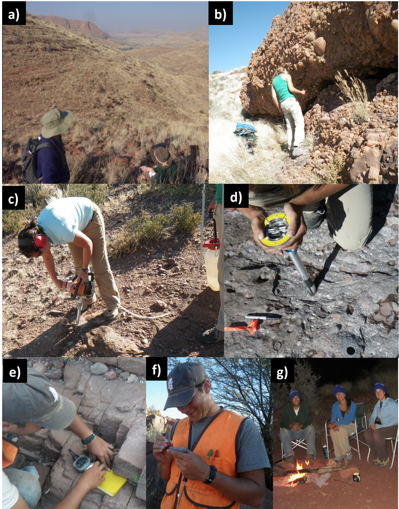
Figure 4: Elements of field sampling: a) Surveying for potential outcrops on Farm Aruab. b) Marking samples to drill at JK1203. c) Drilling cores at JK1201. d) Orienting cores with orienting device at JP1150. e) Taking bedding measurements at JK1206. f) Labeling samples at JK1205. g) Getting back to camp near JK1206.
