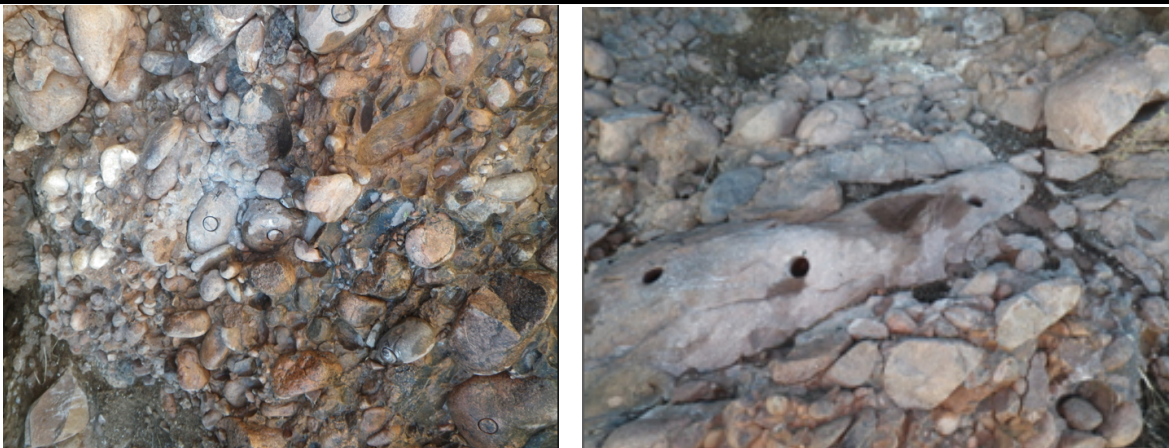
Figure 9: Descriptions of conglomerate test sites from field seasons 2011 and 2012. Images of clasts and matrix sampled at JK1203. 2.5 cm core holes for scale.
