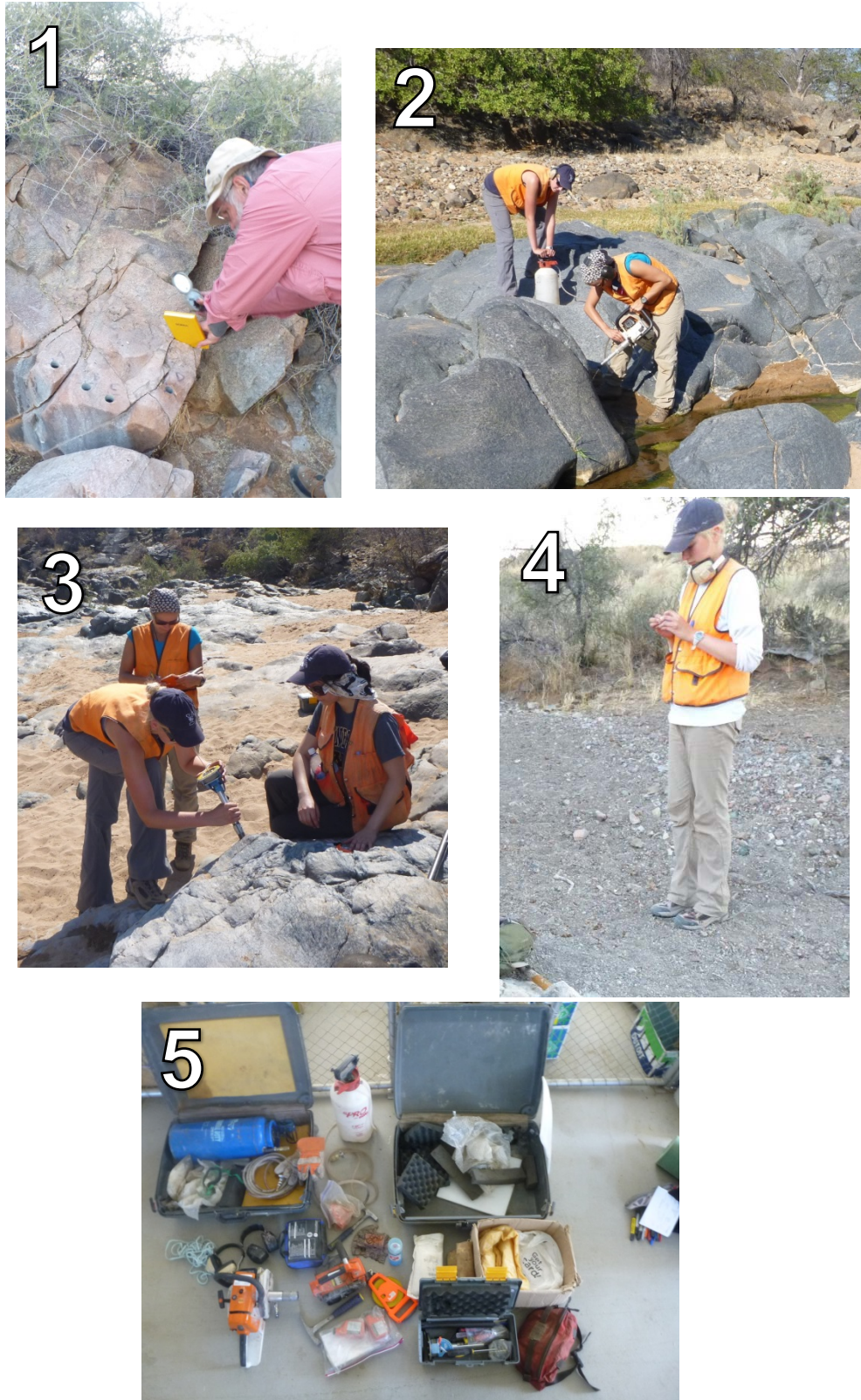
Figure 6: Components of sampling during the 2014 field season in Namibia: 1) Taking bedding measurements (can be done before or after drilling), 2) Drilling cores after marking sample locations, 3) Orienting cores, 4) Removing, labelling, and wrapping cores, 5) Inventory of field equipment carried to each site.
