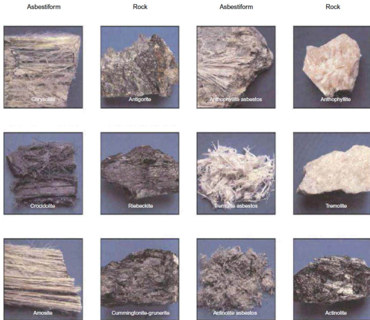
Figure 4. Hand specimens of the six asbestos minerals and their non-fibrous counterparts (Strohmeier et al, 2010).
