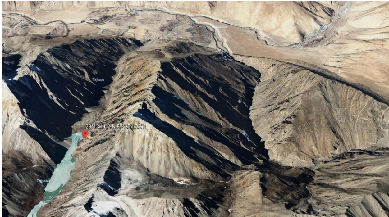
Figure 15. Google Earth imagery showing a potential PHS site under S2 southwest of Yamdrok Lake. The site's quality is good, with a head of 771m and a head to distance ratio of 0.15. The feasibility score is 7.4.
