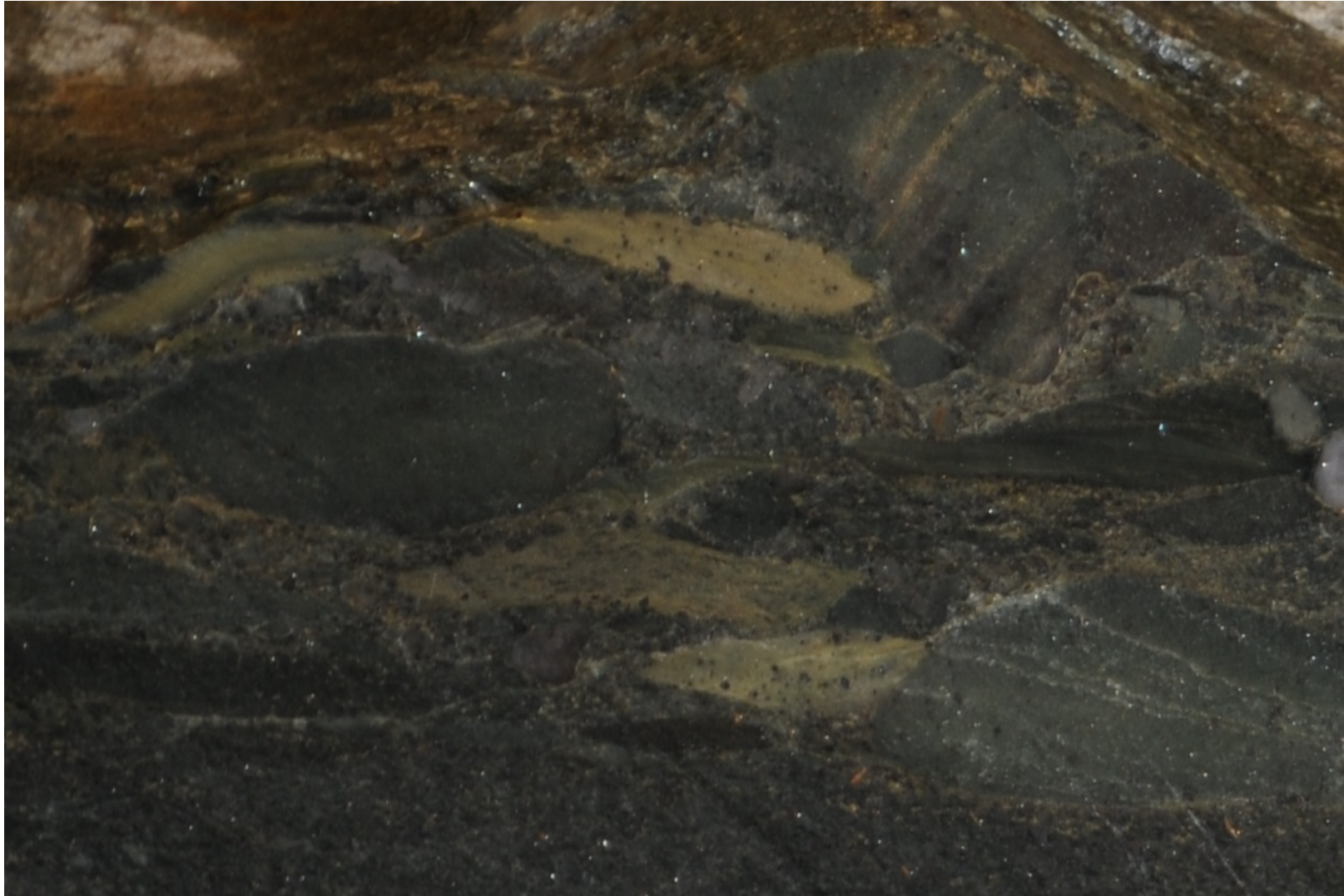
Figure 6b - Magnetite overgrowths within cobble interiors and other pressure solution relicts. Note the varied lithology
